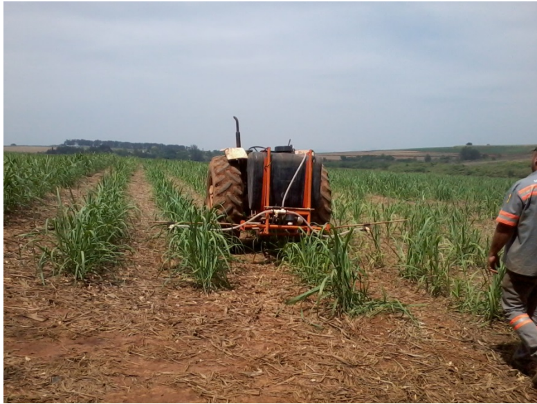
Figure 2. Tractor mounted sprayer used to apply UAN.
