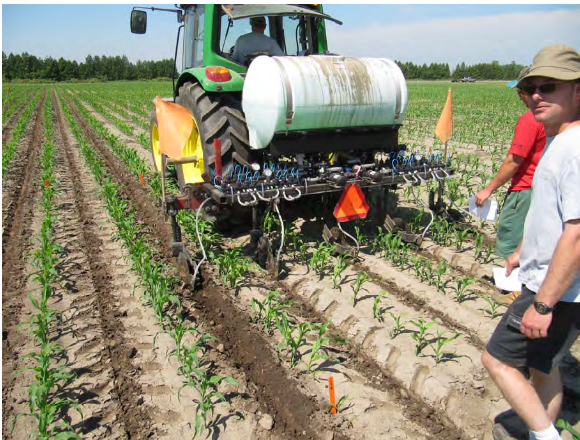
Figure 1. Sidedressing N in project using custom-built variable rate applicator.
