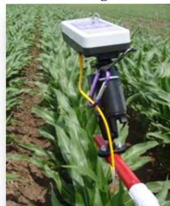
Figure 3: RapidSCAN CS-45 Handheld Crop Sensor scanning corn.
