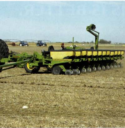
The John Deere row crop planter seeding into alfalfa sod. PHOTO COURTESY OF AGTECH CENTRE
