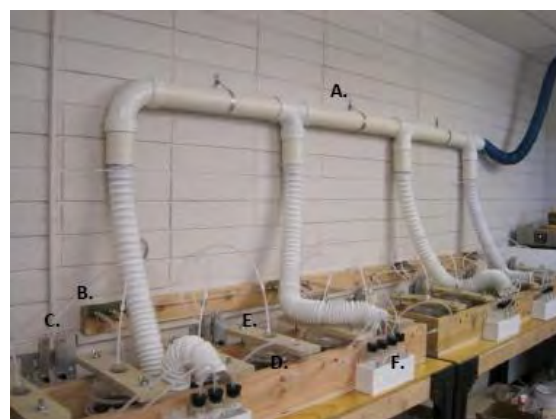
Figure 1: Picture of laboratory chamber system. A. Ventilation system B. Steel Manifold C. 10 L/min flow meter D. Sample Chamber E. Reinforcing 2x4 F. Acid Traps
