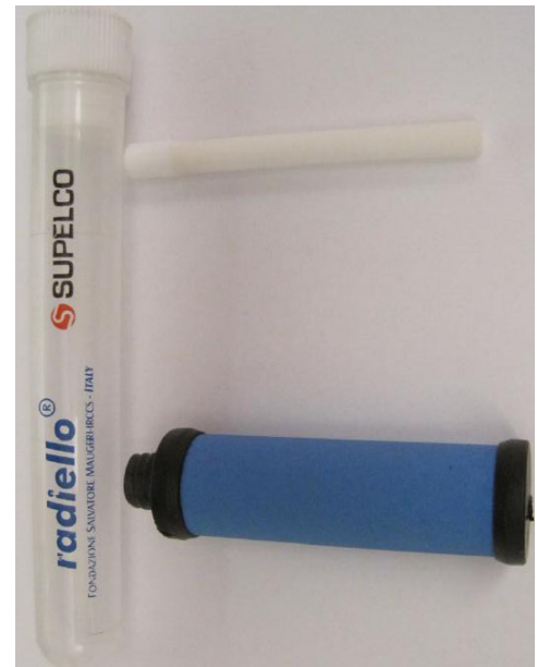
Image 1. Complete Radiello setup with the blue diffusive resistant body, plastic sample container, and phosphorous acid-impregnated polyethylene adsorbing cartridge.
